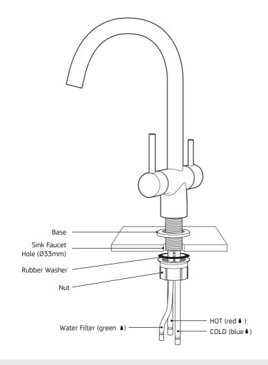
Note: It is important to flush out the supply pipes to the mixer before connecting the flexible hoses with the initial installation, so no foreign matter can enter into the cartridges.
